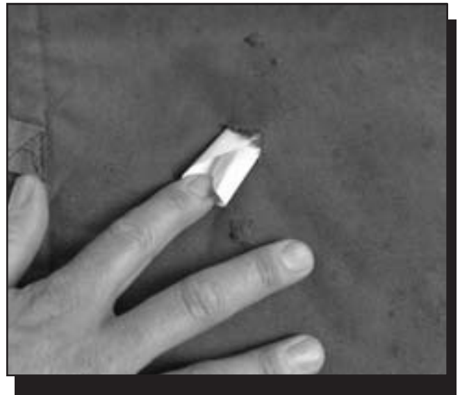
Figure 6—Use paper to prevent Seam Grip patching adhesive from adhering to the protective pad.
