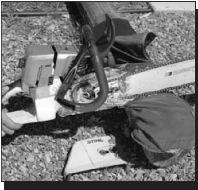
Figure 2—Kevlar fibers jam the chain saw's drive sprocket, stopping the chain saw and preventing injuries.
