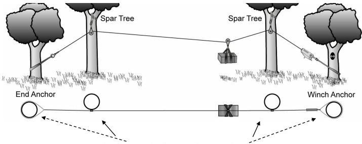
The distance a load moves is between the spar trees.
