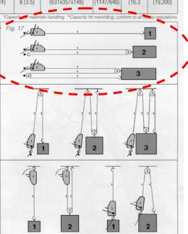
\_ \_ \_ How to set up a 2-1 or 3-1 pull
