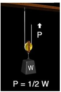
hold up the pulley in this example is 1/2 the weight and the mechanical advantage of this system is 2; Mechanical Advantage in this example is the weight (output force) divided by 1/2 the weight (input force).
