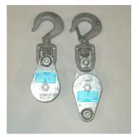
**Snatch blocks** are helpful for building systems to move materials. "Snatch" means that the side of the block will open to accept a line. Snatch blocks are used to build mechanical advantage, change pulling directions, hang highlines from trees and roll loads along a high line.
