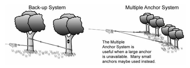
When the available anchor points appear to be small or questionable, use multiple anchor points. It pays to do the best job possible with the anchors. *Winch anchor failure is likely to hurt someone.*
