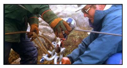
Limit" marked on many products is 1/5 of the breaking strength of the part. Griphoist® machine that produces 2000 pounds of tension needs an anchor sling rated at 2000 pounds WLL (breaking strength of 10,000 pounds). A 4000 pound WLL snatch block (breaking strength of 20,000 pounds) is certainly OK for lifting a 500 pound boulder.
